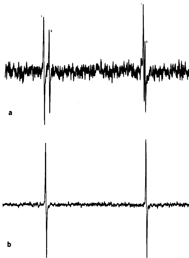
Figure 1. ESR spectra: (a) free (1) and complexed (2) dicarboxymethyl radicals in [\text{HClO}_4] = 0.84 \text{ M} , [\text{Ce}(\text{ClO}_4)_4] = 3 \times 10^{-2} \text{ M} and [\text{MH}] = 0.3 \text{ M} under steady flow; (b) free dicarboxymethyl radical ( M_1 ) in [\text{H}_2\text{SO}_4] = 0.8 \text{ M} , [\text{Ce}(\text{SO}_4)_2] = 3 \times 10^{-2} \text{ M} , and [\text{MH}] = 0.3 \text{ M} . Modulation frequency = 12.5 kHz.
